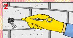
After each brushing cycle clean the hole with a vacuum or blow-out pump or with a compressor. Important! An oil free compressed air line must be used.
