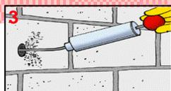
Gun (approx. 2 trigger pulls) until a uniform grey appearance and consistency is obtained, through the mixing nozzle. Do not use unmixed material!
